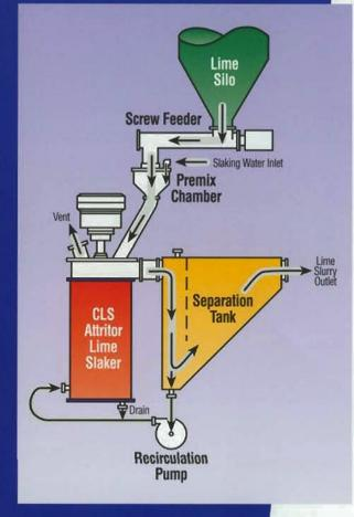
The patented CLS Attritor Stirred Vertical Ball Mill Lime Slaker has been operating successfully in power generating plants for flue gas desulphurization (FGD). The Attritor will slake the lime as well as grind the inert grit, eliminating grit separation and disposal problems.
